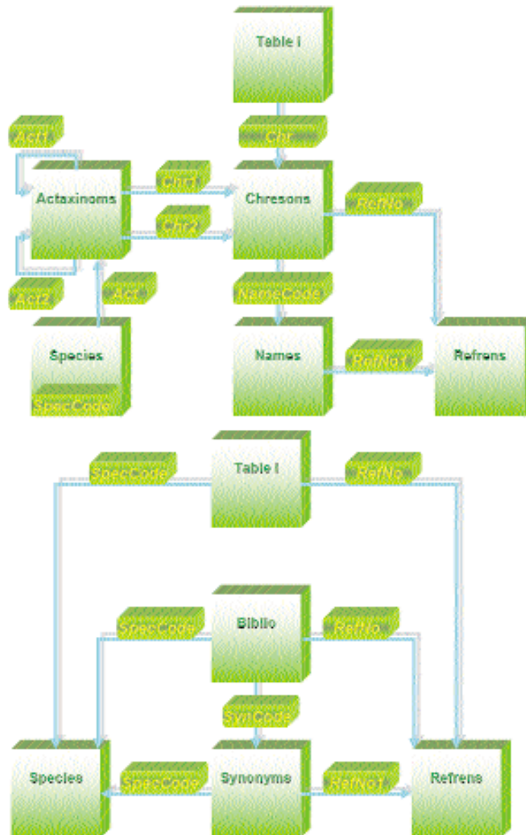
Figure 1 Possible new structure (upper) using the potential taxon concept (here under the name Chresons), compared to the current structure (lower). The synonymies are recorded in the table Actaxinoms, whereas the table Names is a simple repository of words used as names (without author)
